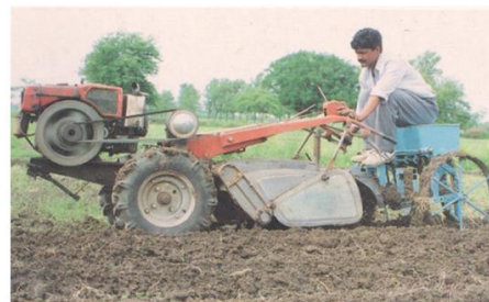
Fig 3: Power tiller operated till-plant machine
