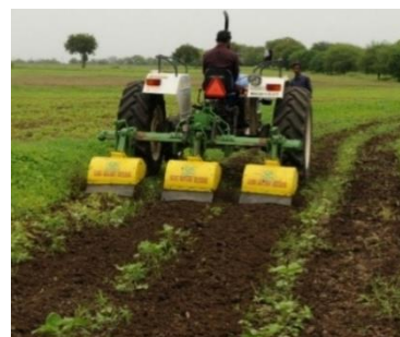
(b) Tractor operated rotary weeder
