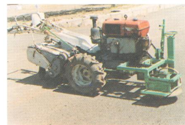
Fig 10: Power tiller operated tree felling machine
