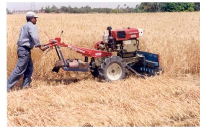
Fig 7: Power tiller operated vertical conveyor reaper
