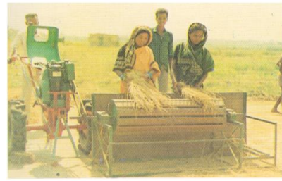
Fig 8: Power tiller operated hold on type thresher
