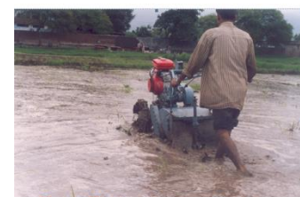
Fig 2. CIAE light weight power tiller during puddling operation
