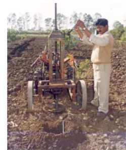
Fig 9: Power tiller operated auger digger
