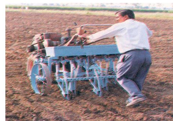
Fig 4: Power tiller operated seed cum fertilizer drill
