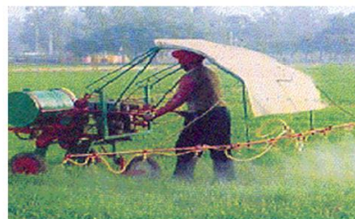
Fig 5: Power tiller operated boom sprayer
