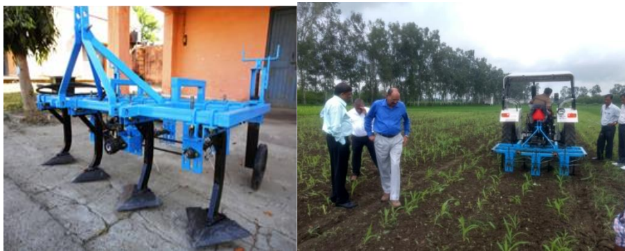
Fig.4: Prototype of three row inter and intra row weeder and field test of weeder in maize field
