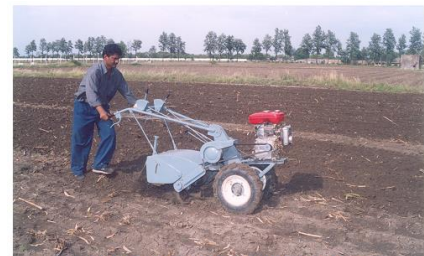
Fig 1. CIAE light weight power tiller during rotatilling operation
