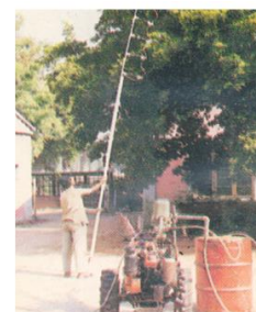
Fig 6: Power tiller operated tall tree sprayer
